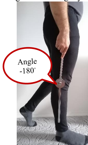
Figure 3.b. Measuring with the mechanical goniometer
