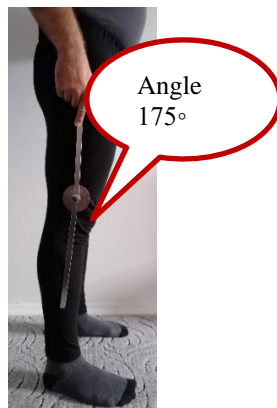
Figure 7.b. Measuring with the mechanical goniometer
